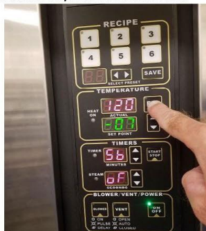
PRESS AND HOLD F/C TO ACCESS PARAMETERS
